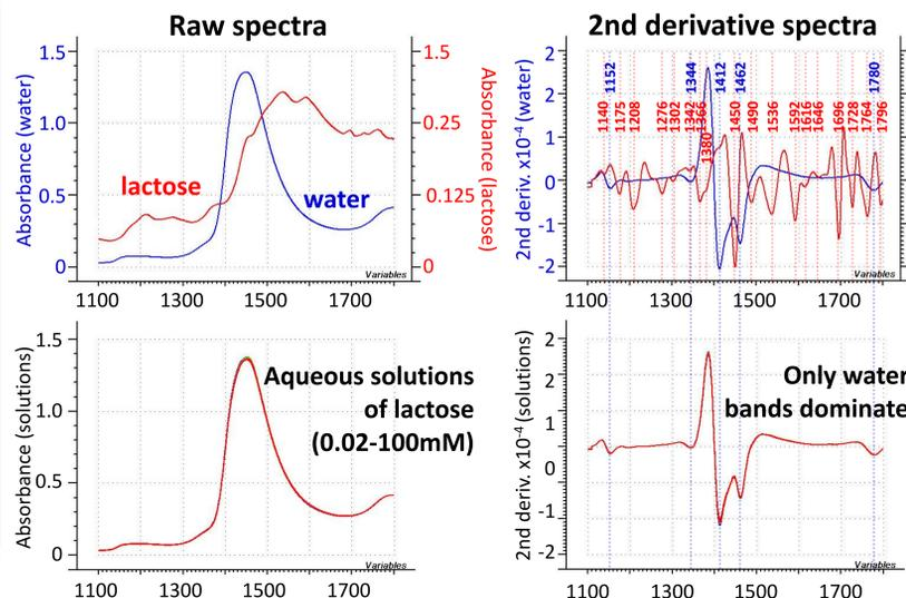
Signals of lactose can hardly be detected in low concentration solutions. Subtraction of water spectrum from those of the lactose solutions reveals the spectral differences of the different concentrations.
