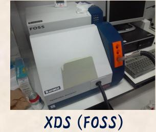
Wavelength: 400-2500 nm Step: 0.5 nm Module: Optiprobe Analyzer Mode: Transflectance Pathlength: 1.0 mm
