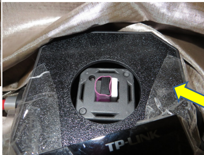
Temperature controlled cuvette holder (1mm cuvette inside)
